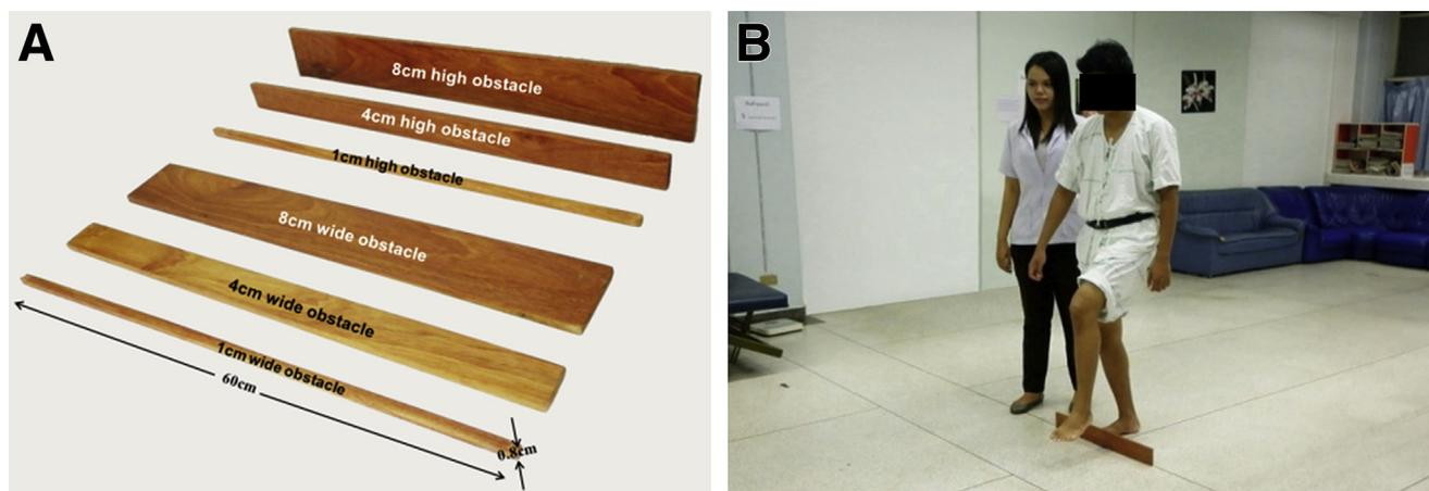
**Fig 1** Obstacles used and testing protocol. (A) Wooden obstacles of 6 sizes. (B) An obstacle crossing task (for 8-cm-high obstacle).
